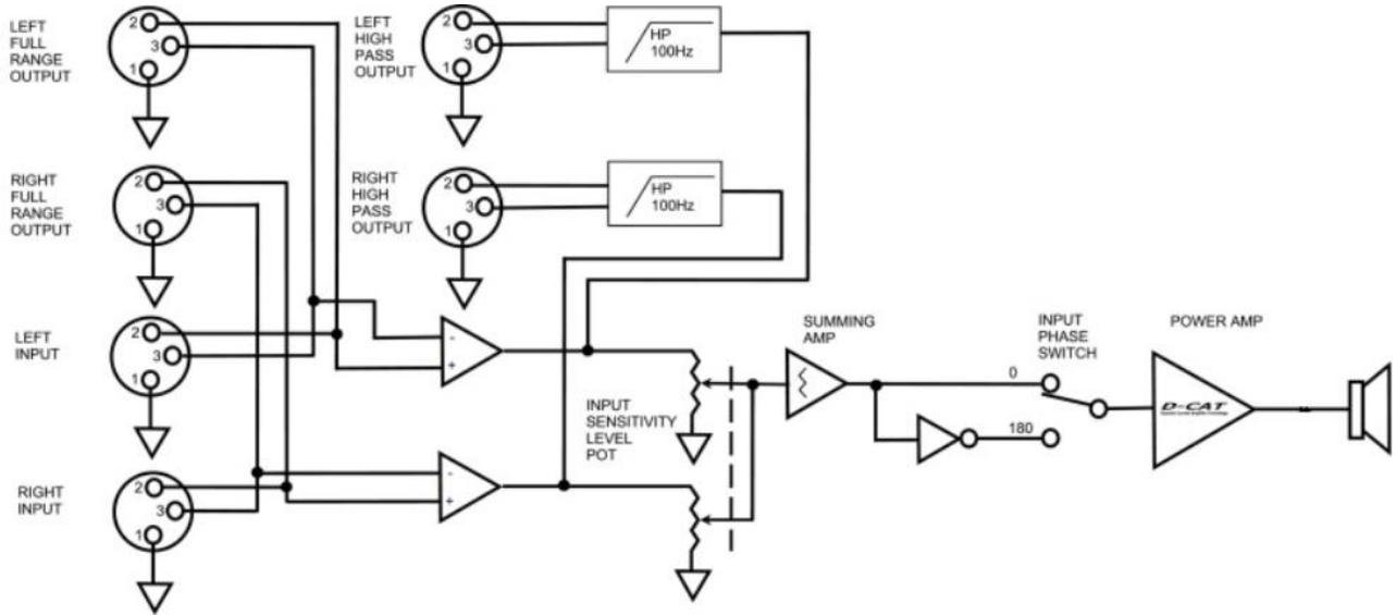
The ISP Sub Series has balanced XLR and inputs and outputs configured to AES standards (Audio Engineering Society). These connections are connected in a loop through configuration from the inputs to the full range outputs and will accept a balanced line-level input. The standard phase configuration is that pin 2 is (+), pin 3 is (-), and pin 1 is shielded ground on the XLR.
