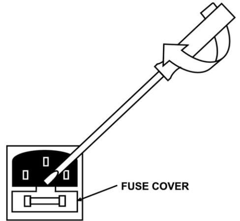
2. After replacing the fuse with another of identical specifications, push the fuse cover module fully back into place, ensuring that the fuse has snapped onto the fuse holder inside the power inlet module.
