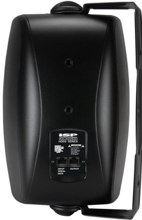
The rear panel includes two RJ45 connectors one for input and one for output. Connect the input to the output connector on a HDDS Master Control Module. A Cat5 cable is used to connect the output connector to another SM652 or to connect to any other ISP Technologies HDDS powered speaker.
