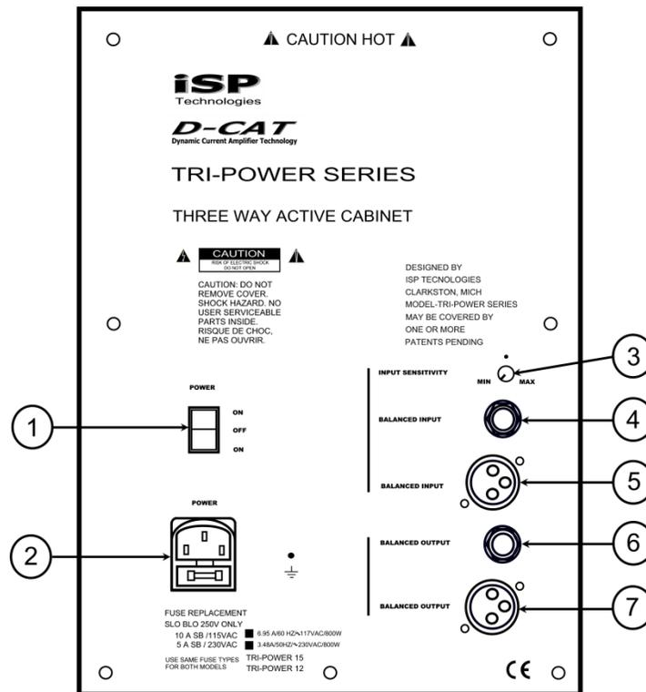
**1. POWER SWITCH**-This switch provides power to the Tri-Power power amp section. This switch is a three-position switch where center is OFF and the outer positions are ON.
