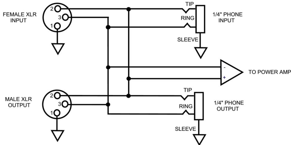
NOTE: IF AN UNBALANCED SIGNAL SOURCE IS USED, THE MALE XLR AND 1/4" PHONE OUTPUTS FOR LOOPING THROUGH TO ADDITIONAL POWERED CABINETS WILL ALSO BE UNBALANCED.
