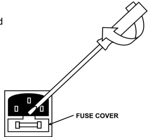
2. After replacing the fuse with another of identical specifications, push the fuse cover module fully back into place, ensuring that the fuse has snapped onto the fuse holder inside the power inlet module.
